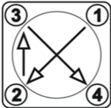
Figure 2 - Screw tightening procedure
